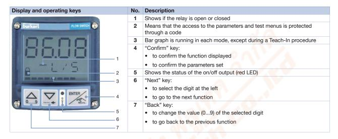
The device can be calibrated by means of the K-factor (conversion coefficient), or via the Teach-In function. User adjustments, such as engineering units, output, filter, bargraph are carried out on site.
