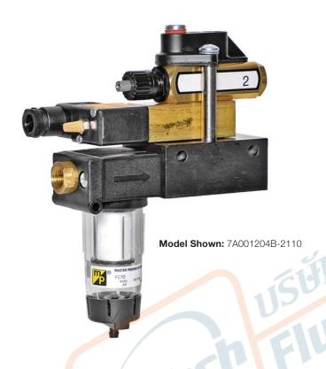
The electronically controlled multiple-point lubricator has a 3-way solenoid-controlled valve to produce the actuating signals for the Servo-Meters (up to four may be used.). This allows lubrication control to be interfaced with other system electronics, so that the frequency of oil injection is under precise control.
