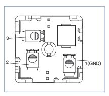
The inverter electronics Type 2508 IN is used to control impulse valves with reverse polarity control by means of 3 control signals (ON, OFF and GND). The switching occurs by reversing the polarity of the valve supply voltage.
