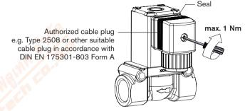
Cable plug can be rotated 4 x 90°.
