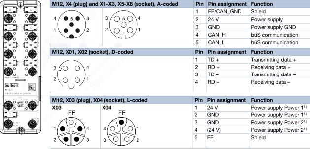
1) The power supplies Power 1 and Power 2 are internally connected.
