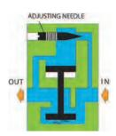
When inlet pressure is removed, the exhausting downstream air pressure keeps the inlet poppet open until the downstream pressure drops by approximately 90 percent. The remaining pressure is exhausted via the delay orifice. An upstream exhaust port (as in a separate lockout valve) is needed for proper operation.
