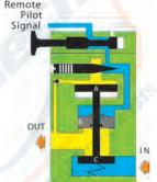
Lockout open and pilot signal applied. Pilot air forces piston B downward to close exhaust port. Pilot air also flows past the metering pin, opens the ball check, and slowly pressurizes the outlet line. Pressure is also building up on piston A.
