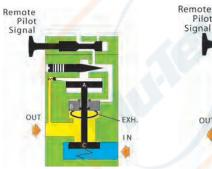
Lockout open and no pilot signal. Inlet air is blocked by inlet poppet C. Any downstream pressure forces sliding piston B upward. This opens the exhaust port and vents the downstream air.
