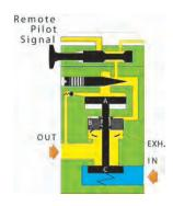
Lockout closed. At any time the lockout handle can be pushed inward, closing off the flow of pilot air. Pilot air above pistons A and B is then vented through the exhaust port. Piston A moves upward closing inlet poppet C. Sliding piston B moves upward opening the exhaust port and venting the downstream line.
