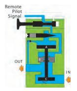
When the pressure on piston A reaches 50% of inlet pressure, the piston is forced downward, opening inlet poppet C. Inlet air now flows freely to the outlet port.
